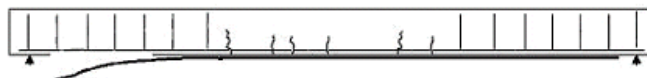
(c) Ripping off of concrete cover, with FRP still bonded to the concrete
