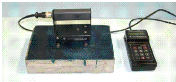
Olson Instruments impact echo tester.
