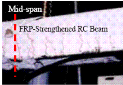
(a) Rupture of FRP
