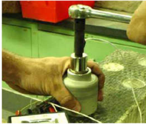
Pull-off tester; destructive testing.
