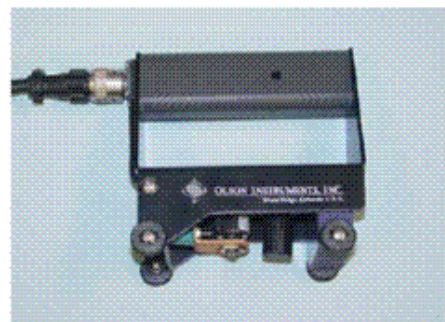
Impact echo tester modified with air coupled receiver.
